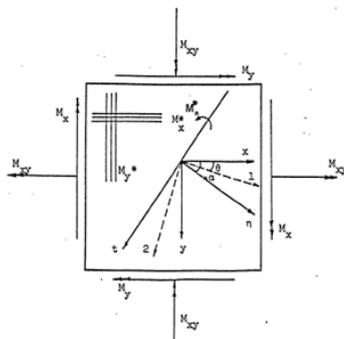
Figure (3.2) Element with Orthogonal Reinforcement
