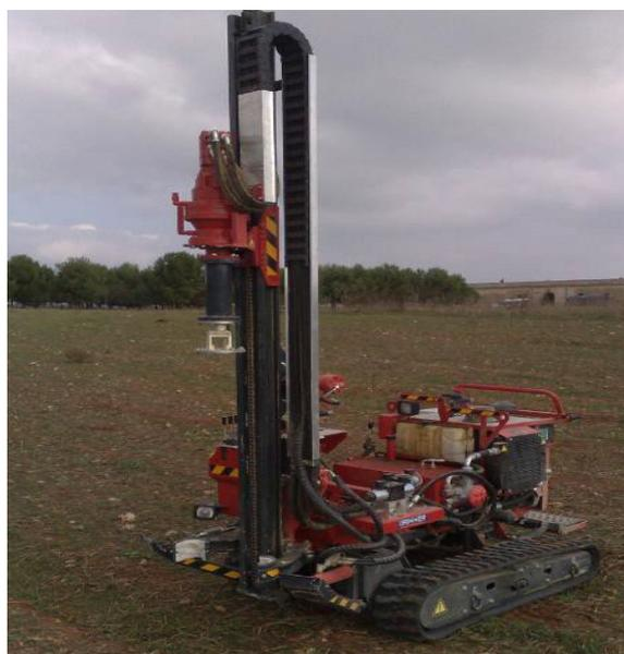
**Figura 34 – MACCHINA BATTIPALO PER INFISSIONE PALI**
