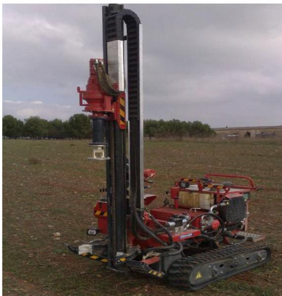
**FIGURA 35 – MACCHINA BATTIPALO PER INFISSIONE PALI.**
