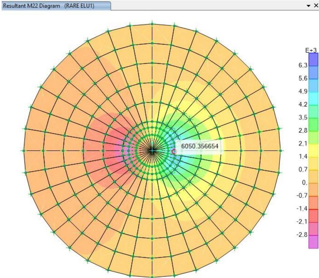
**Figura 9-5: Momento Massimo M<sub>22</sub> Normal SLU 1 [kNm/m]**
