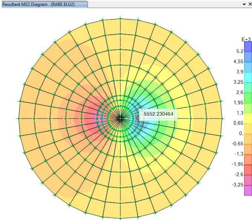
**Figura 9-6: Momento Massimo M<sub>22</sub> Normal ELU 2 [kNm/m]**
