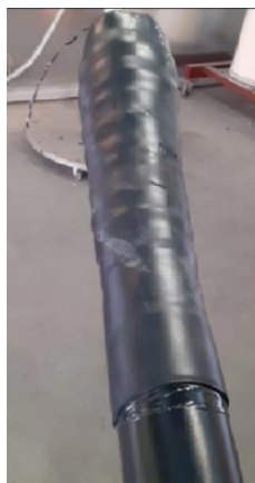
Figure 4-6 – WTG/OSS Cable Connection System (Typical)
