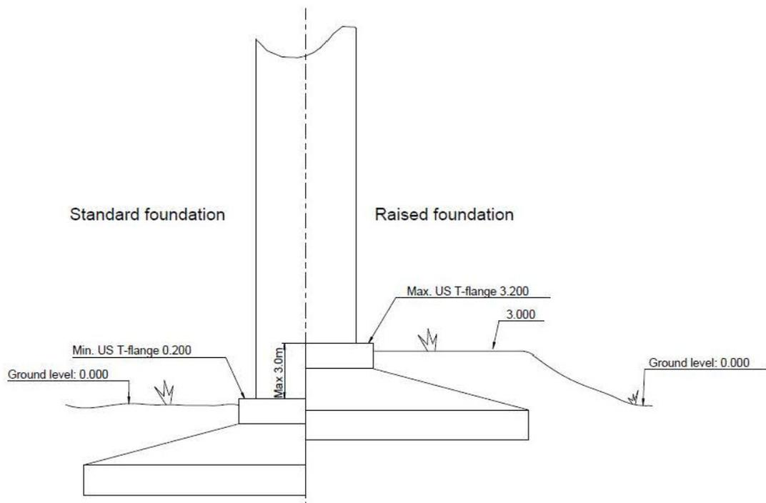
Figure 1-1 Tower and Foundation interface
