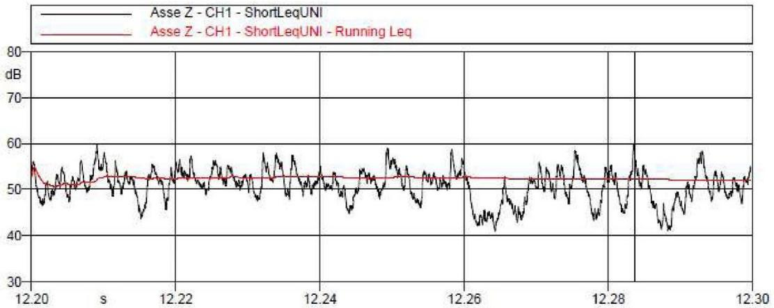
**SINTESI LIVELLI ASSE Z** LwUNI9614 = 52.1 dB    Lw\_max = 59.9 dB    Lim\_UNI9614 = 80.0/77.0 dB
