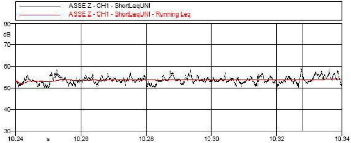
SINTESI LIVELLI ASSE Z LwUNI9614 = 53,9 dB Lw\_max = 59,7 dB Lim\_UNI9614 = 80,0/77,0 dB
