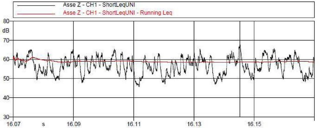
**SINTESI LIVELLI ASSE Z** LwUNI9614 = 58.7 dB    Lw\_max = 67.6 dB    Lim\_UNI9614 = 80.0/77.0 dB
