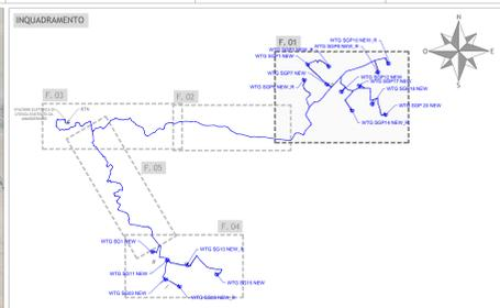
**VERIFICA DISTANZE RISPETTO AD AEROGENERATORI IN PROGETTO (Espressa in diametri - D = 172m)**
