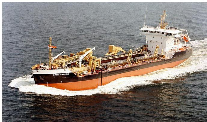
*Figura 4.16: trailing suction hopper dredger*
