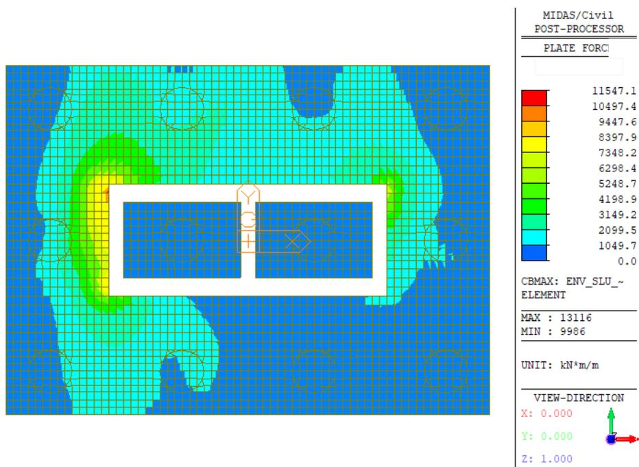
Figura 34 – Wood Armer Moment – Direction1 – Bottom (Involuppo SLU/SLV)
