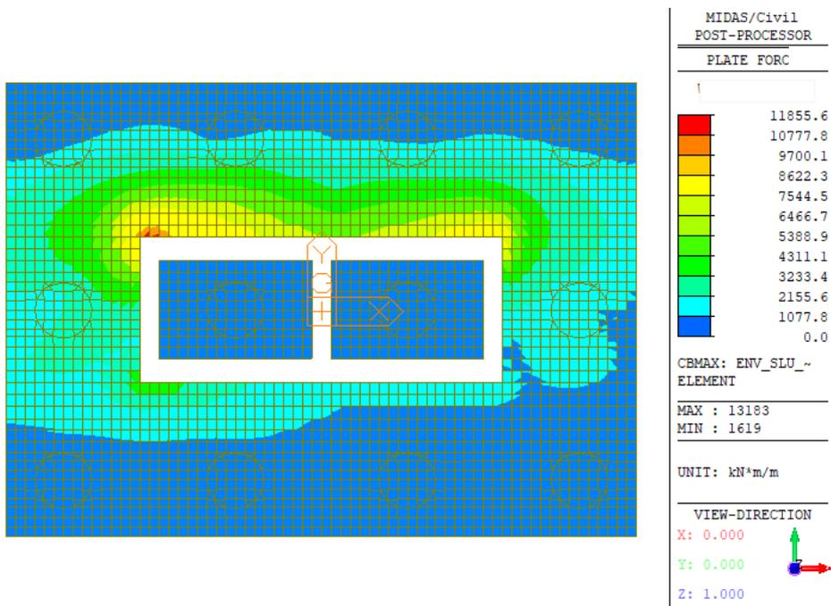
Figura 36 – Wood Armer Moment – Direction 2 – Bottom (Inviluppo SLU/SLV)
