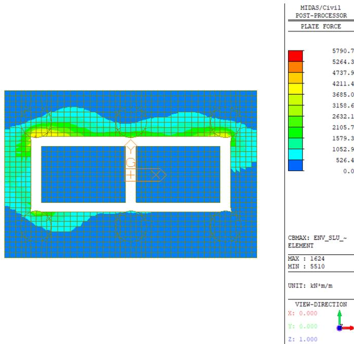
Figura 34 – Wood Armer Moment – Direction 2 – Bottom (Involuppo SLU/SLV)
