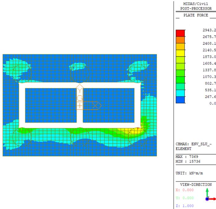
Figura 33 – Wood Armer Moment – Direction 2 – Top (Involuppo SLU/SLV)
