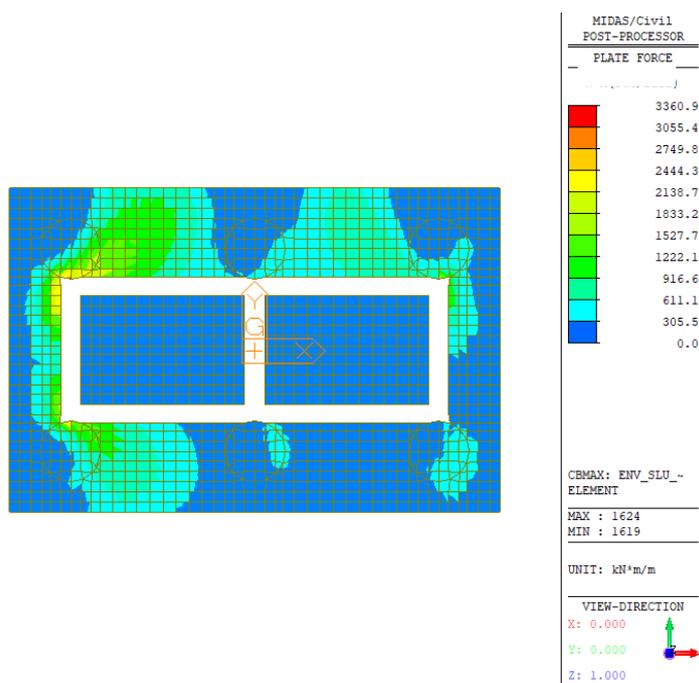
Figura 32 – Wood Armer Moment – Direction1 – Bottom (Inviluppo SLU/SLV)
