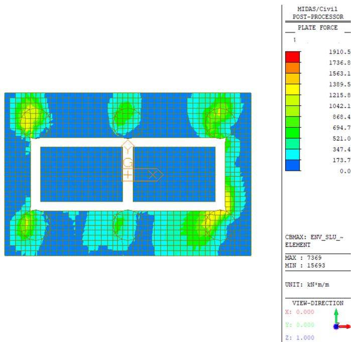
Figura 31 – Wood Armer Moment – Direction1 – Top (Inviluppo SLU/SLV)
