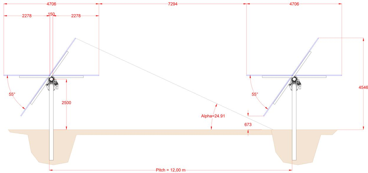
ALTEZZA MODULI SU STRUTTURE MOBILI: Hmin = 0,67 m - Hmax = 4,55 m - Hmedia = 2,61 m
