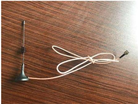
Figure 20, LORA wireless antenna
