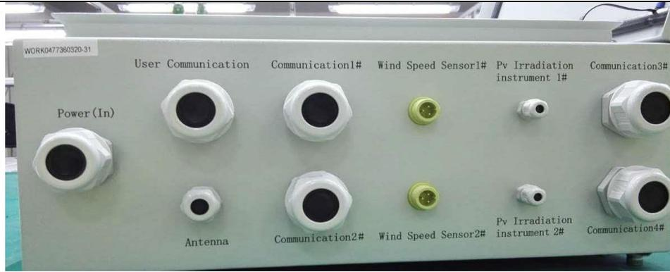
Figure 19, Communication box ports
