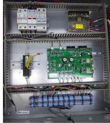
Figure 23, Internal components of the communication box
