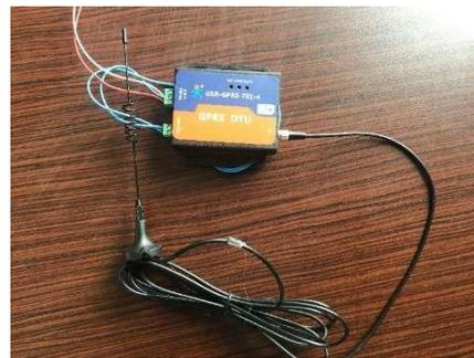
Figure 21, DTU & its Antenna
