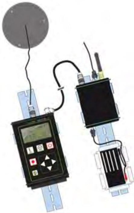
Fig. 1: Batcorder 2.0 with GSM remote control unit
