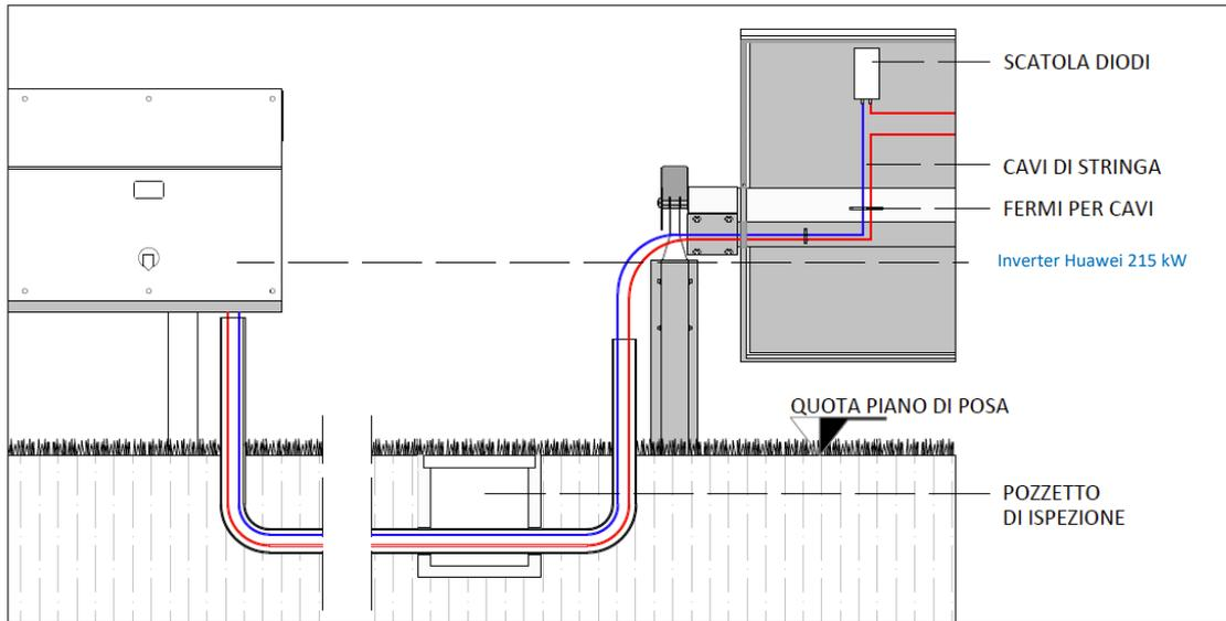
Particolari connessione Inverter Huawei 215 kW
