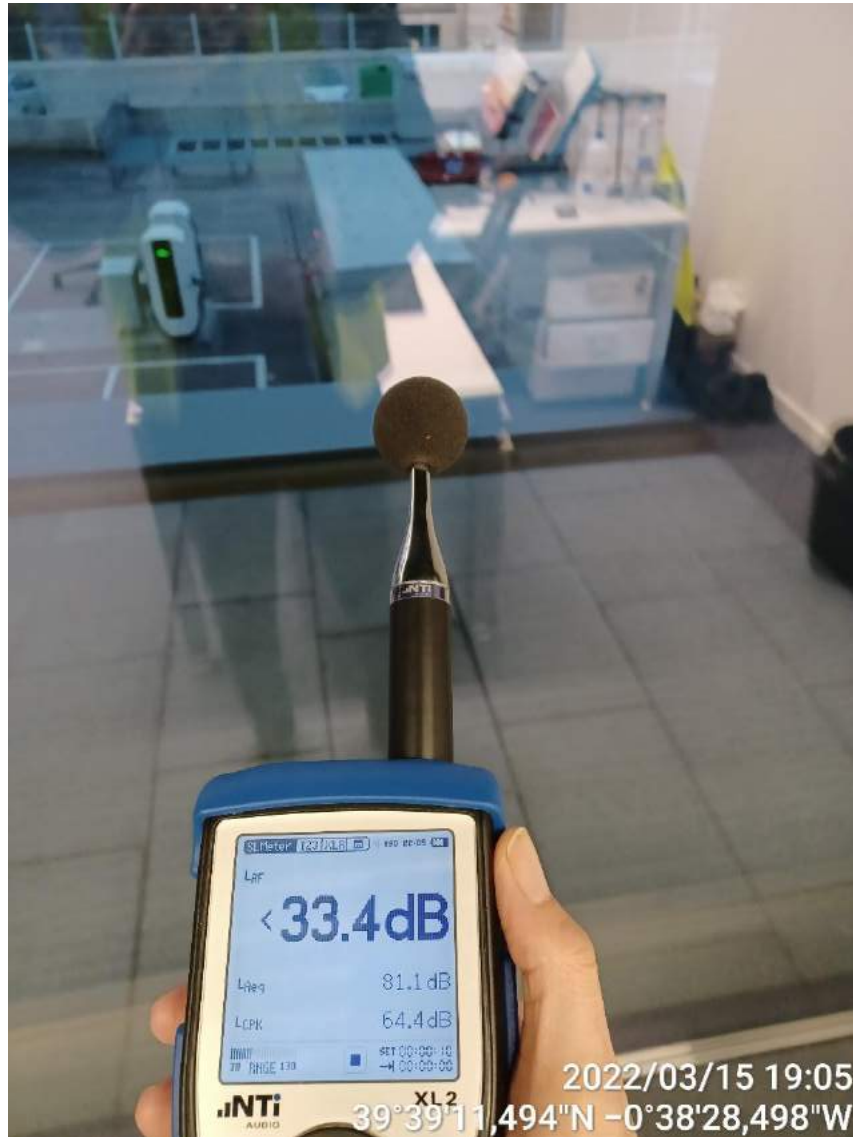
Pic. 2. 30m from the inverter, inside a building.
