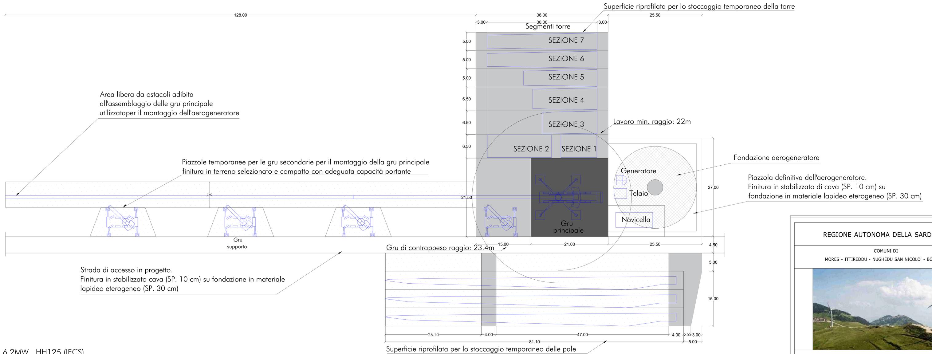
CRANE PAD V162 6.2MW HH125 (IECS)
