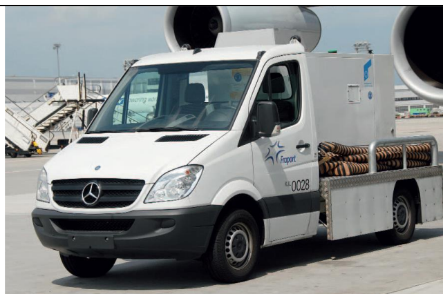
AIR START UNIT
