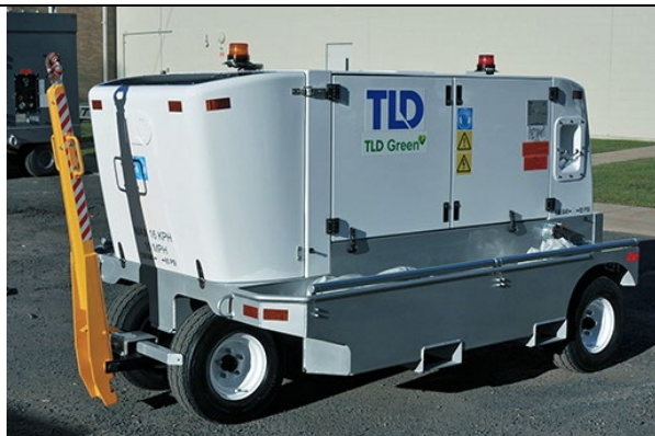
GROUND POWER UNIT 409
