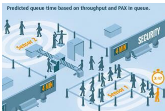
Figura 51 - Passenger Tracking System
