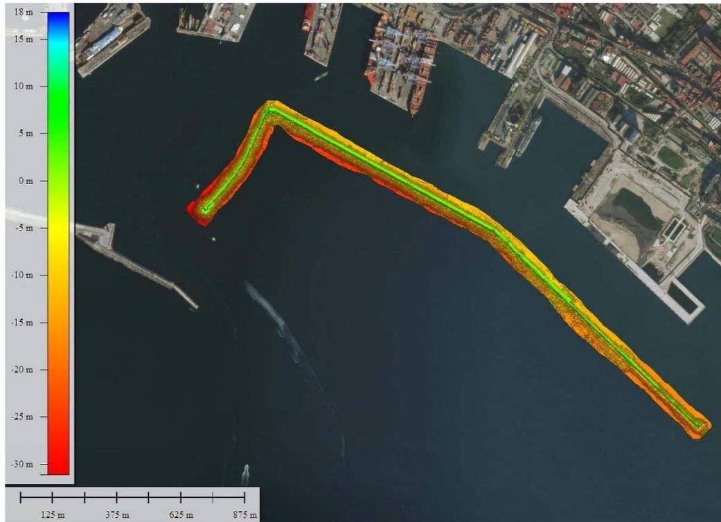
FIGURA 4.1 - DIGA DUCA D'AOSTA E ANTEMURALE THAON DE REVEL – MAPPATURA BATIMETRICA 2021
