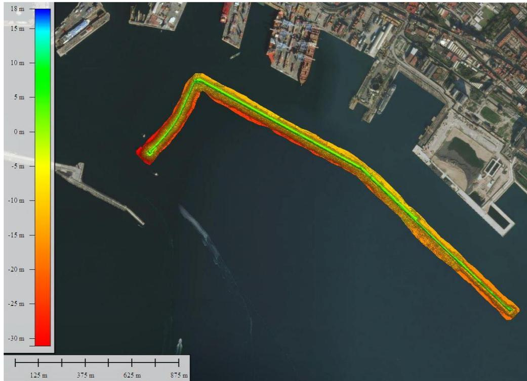
FIGURA 34 - DIGA DUCA D'AOSTA E ANTEMURALE THAON DE REVEL – MAPPATURA BATIMETRICA 2021
