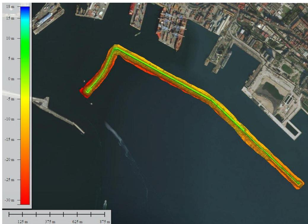
FIGURA 54 - DIGA DUCA D'AOSTA E ANTEMURALE THAON DE REVEL – MAPPATURA BATIMETRICA 2021
