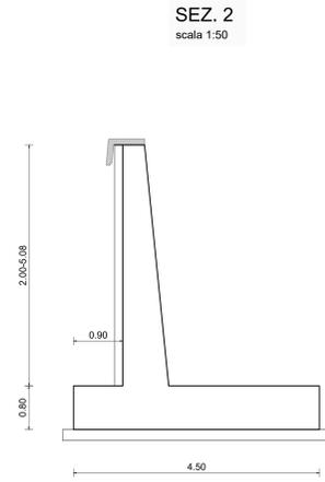
**MURO IN C.A. GA02: INCIDENZA ARMATURE**
