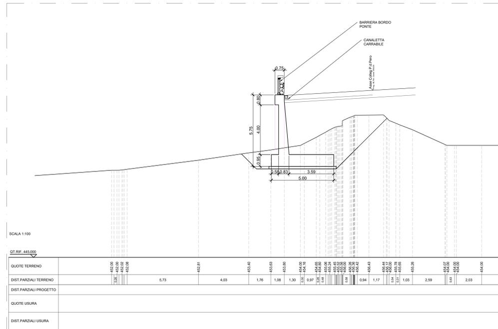
**TIPOLOGICO FASI COSTRUTTIVE MURO IN SCAVO**
