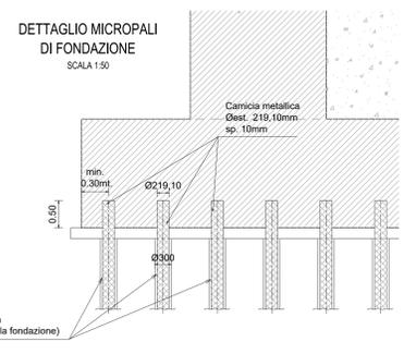
LA CAMICIA METALLICA DEI MICROPALI DI FONDAZIONE E' IN ACCIAIO CLASSE S355 (σ<sub>traccatura</sub> = 219, 10mm - sp. 10mm).
