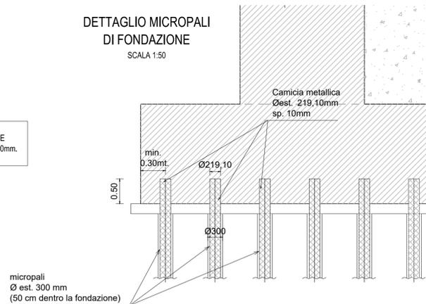
LA CAMICIA METALLICA DEI MICROPALI DI FONDAZIONE E' IN ACCIAIO CLASSE S355: Ø<sub>ESTERNO</sub> = 219,10mm - sp. 10mm.
