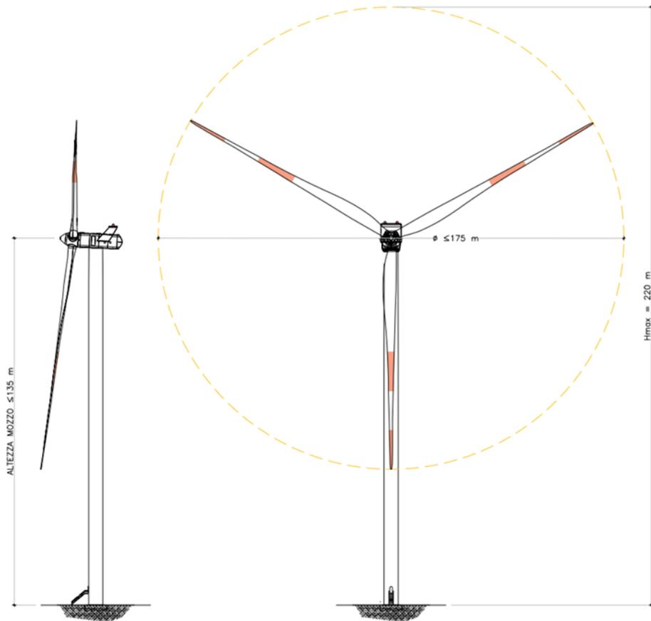
Tip height=220m; hub height<=135m; rotor diameter<=175m;
