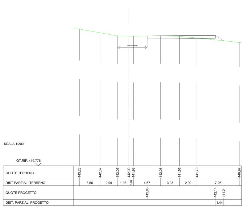
SEZIONE N.: 5 QT. PROGETTO: 443,618 DIST.PROG.: 1082,003 DIST.PREC.: 23,849
