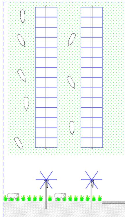
DETTAGLIO (PIANTA E PROSPETTO) SISTEMA AGRIVOLTAICO
