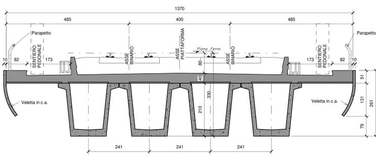
PROSPETTO TIPO IN CAMPATA-Scala 1:50
