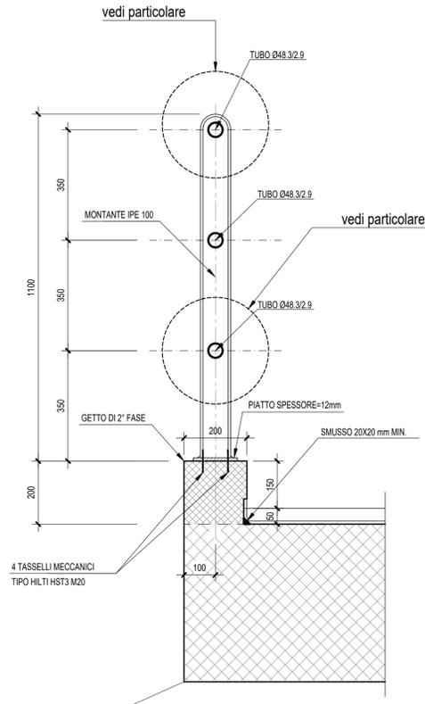
PARTICOLARI PARAPETTO IN ACCIAIO
