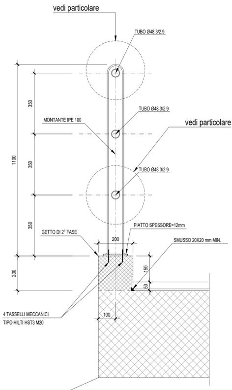
PARTICOLARI PARAPETTO IN ACCIAIO
