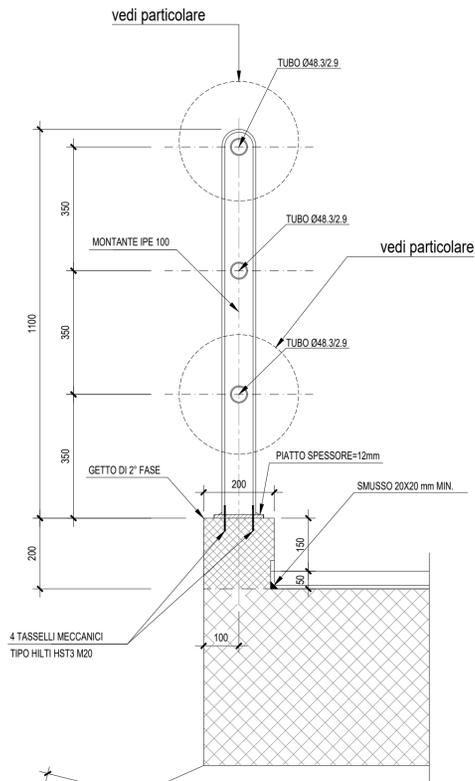
PARTICOLARI PARAPETTO IN ACCIAIO
