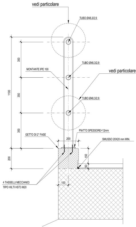
PARTICOLARI PARAPETTO IN ACCIAIO
