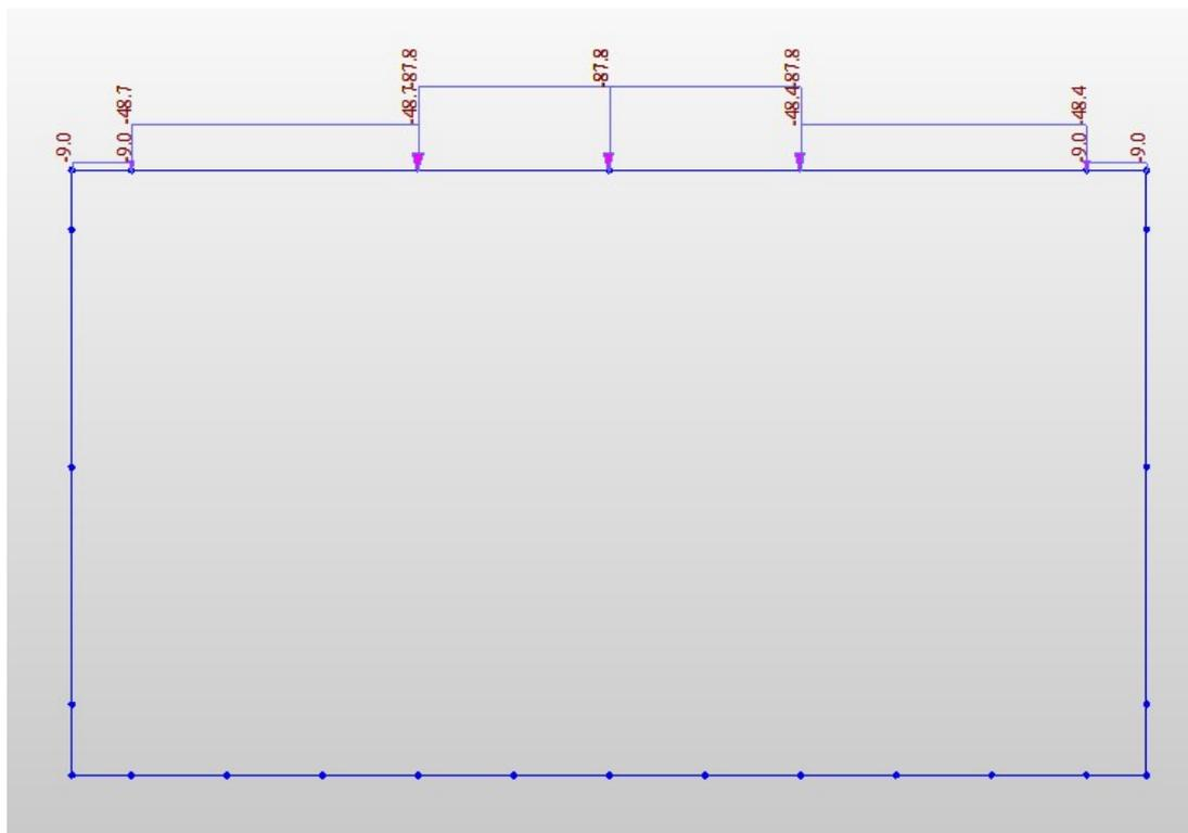
*Fig. 15 – Carico mobile considerate ACC1, sul MIDAS*
