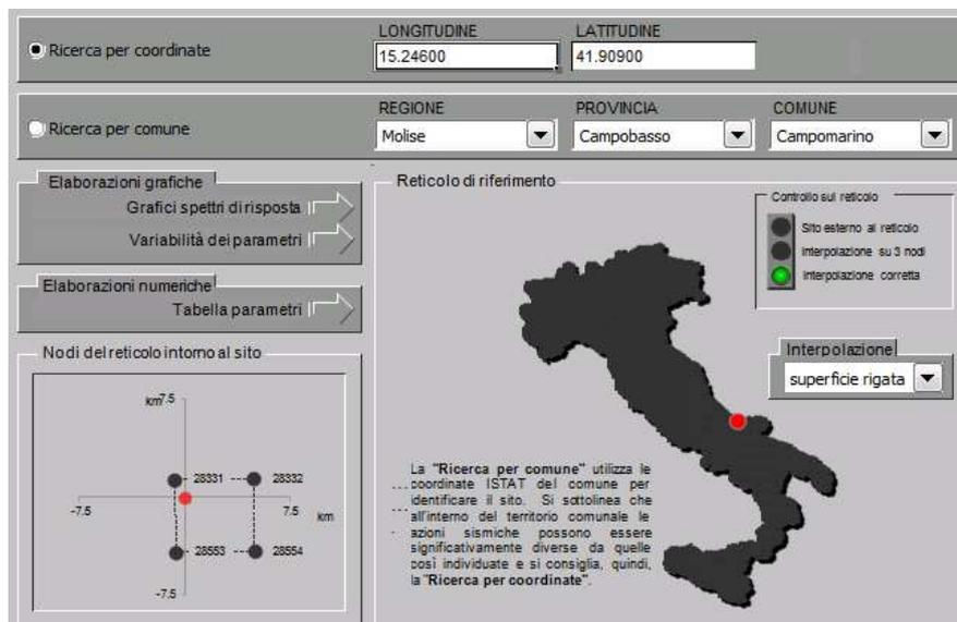
The screenshot displays a software interface for seismic hazard analysis. It features search options for coordinates and comune, a map of Italy with a red dot indicating the site location, and a grid of nodes around the site. The interface includes fields for longitude (15.24600) and latitude (41.90900), and dropdown menus for region (Molise), province (Campobasso), and comune (Campomarino). A legend indicates site status and interpolation methods.
