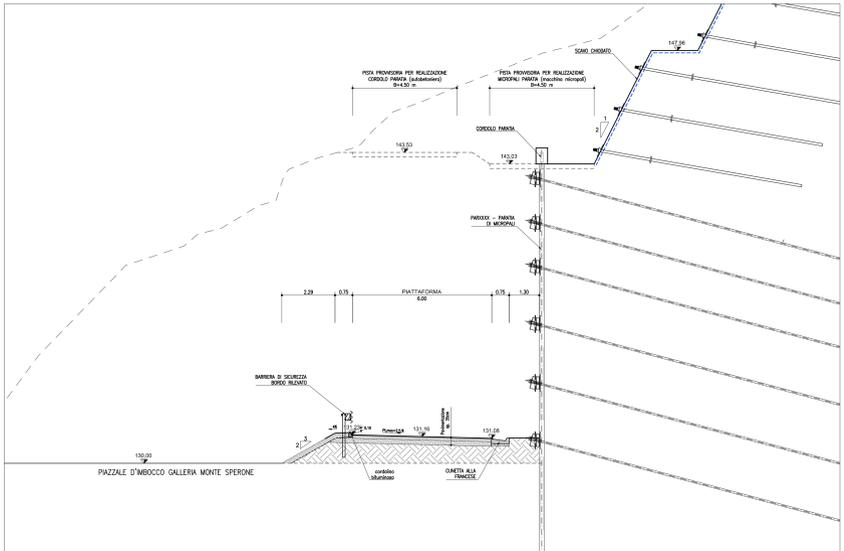
MARGINE ESTERNO IN RILEVATO CON SCARPATA IN TERRA
