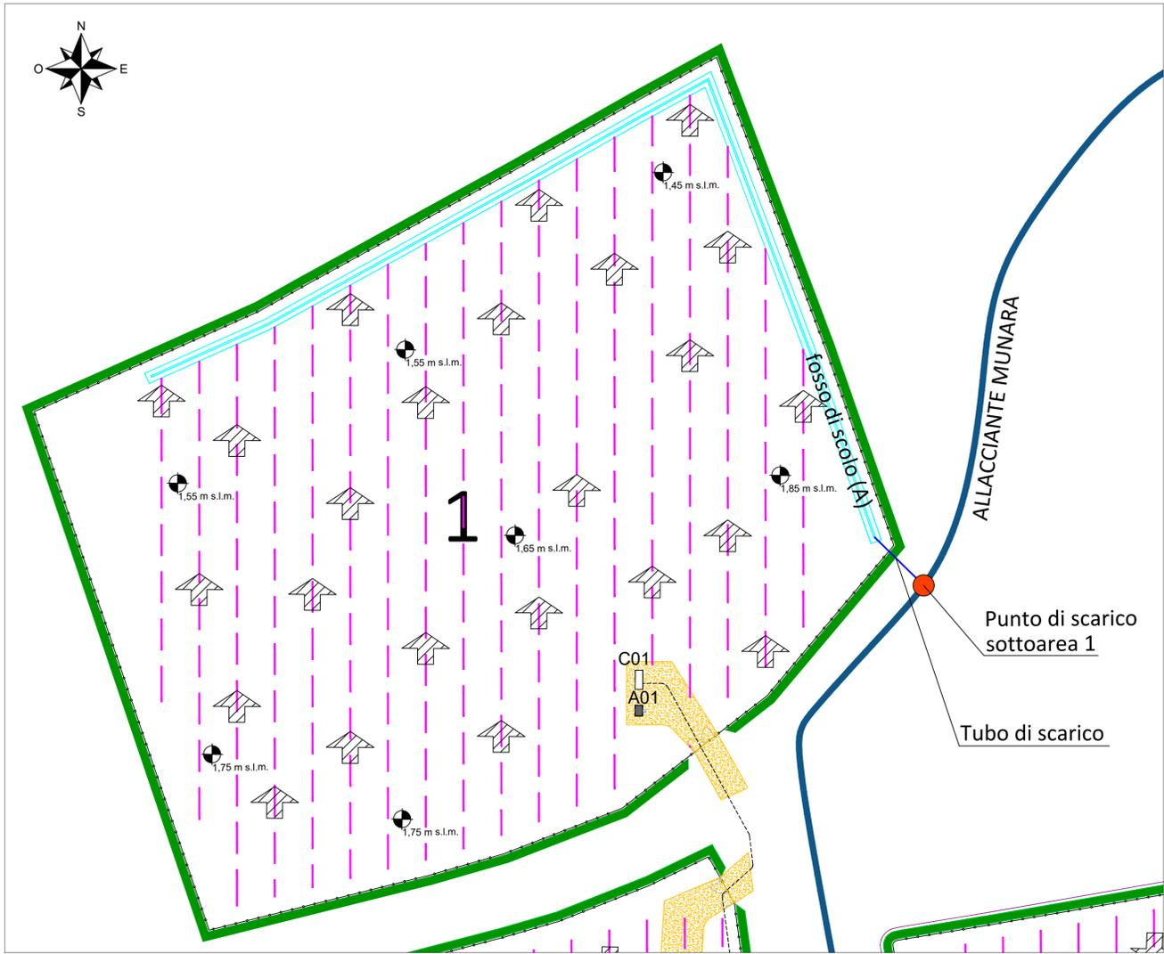
PLANIMETRIA OPERE IDRAULICHE AREA 1 - SOTTOAREA 1 - SCALA 1:1000
