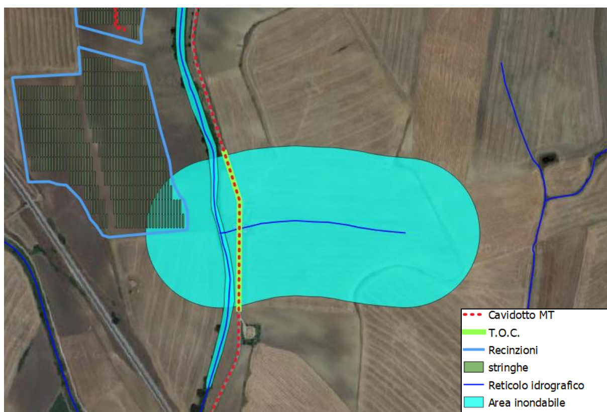
Attraversamento in T.O.C.
