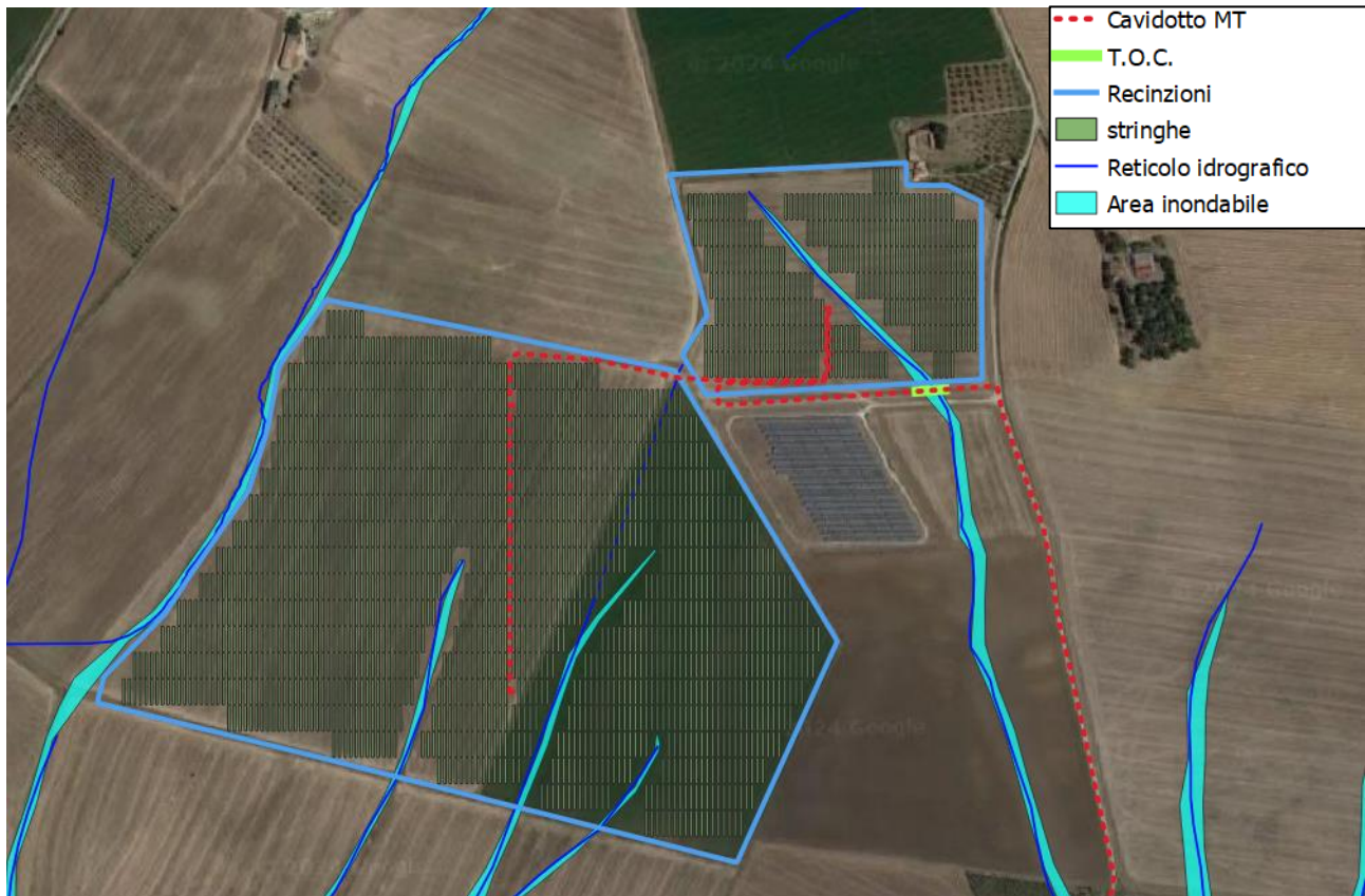
Attraversamento in T.O.C.
