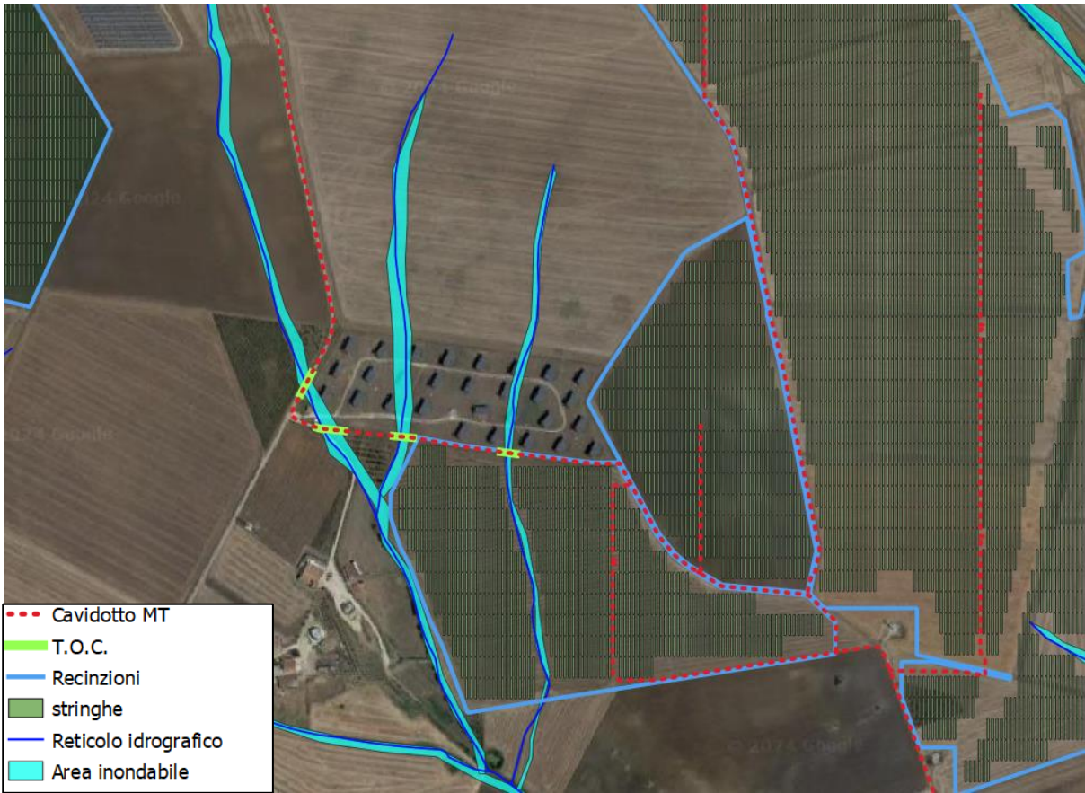
Attraversamento in T.O.C.
