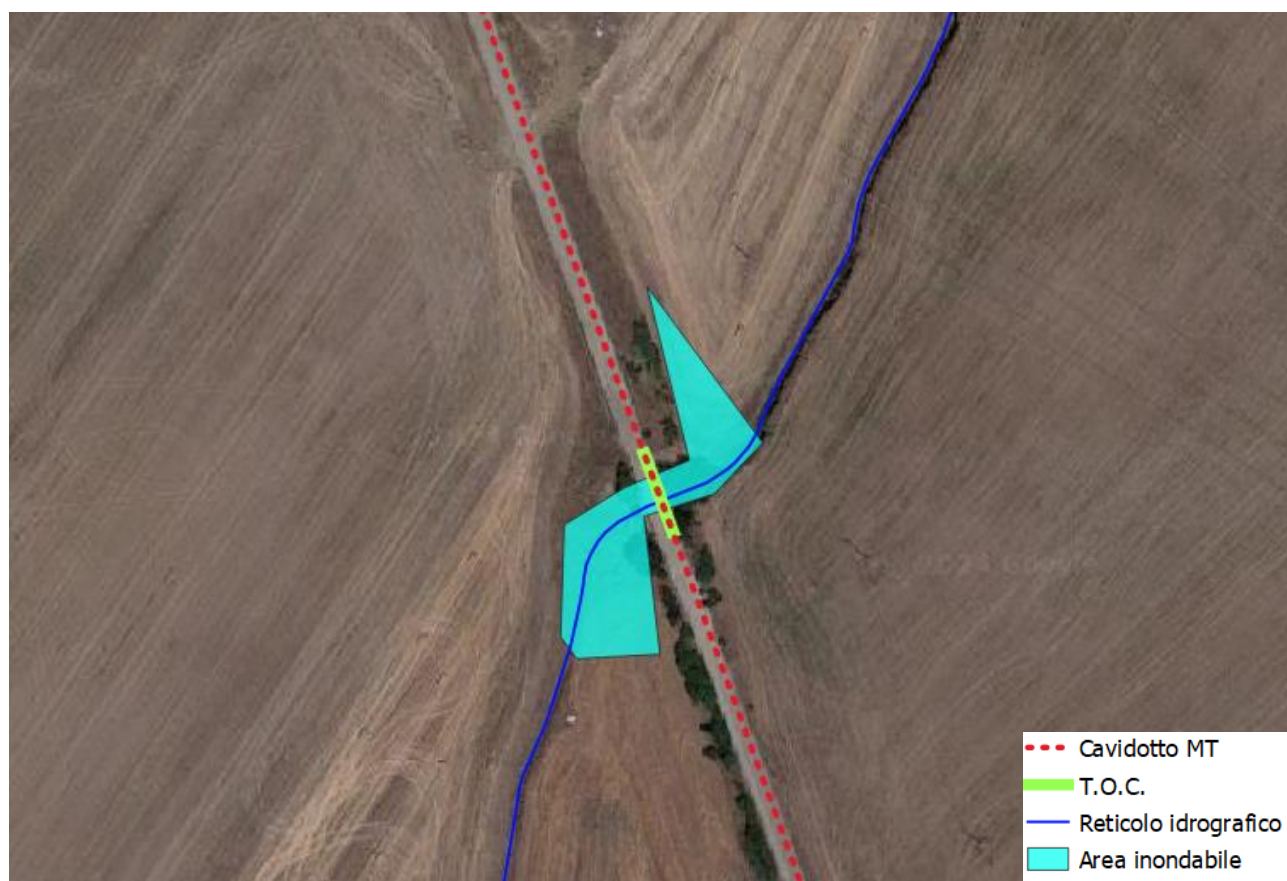
Attraversamento in T.O.C.
