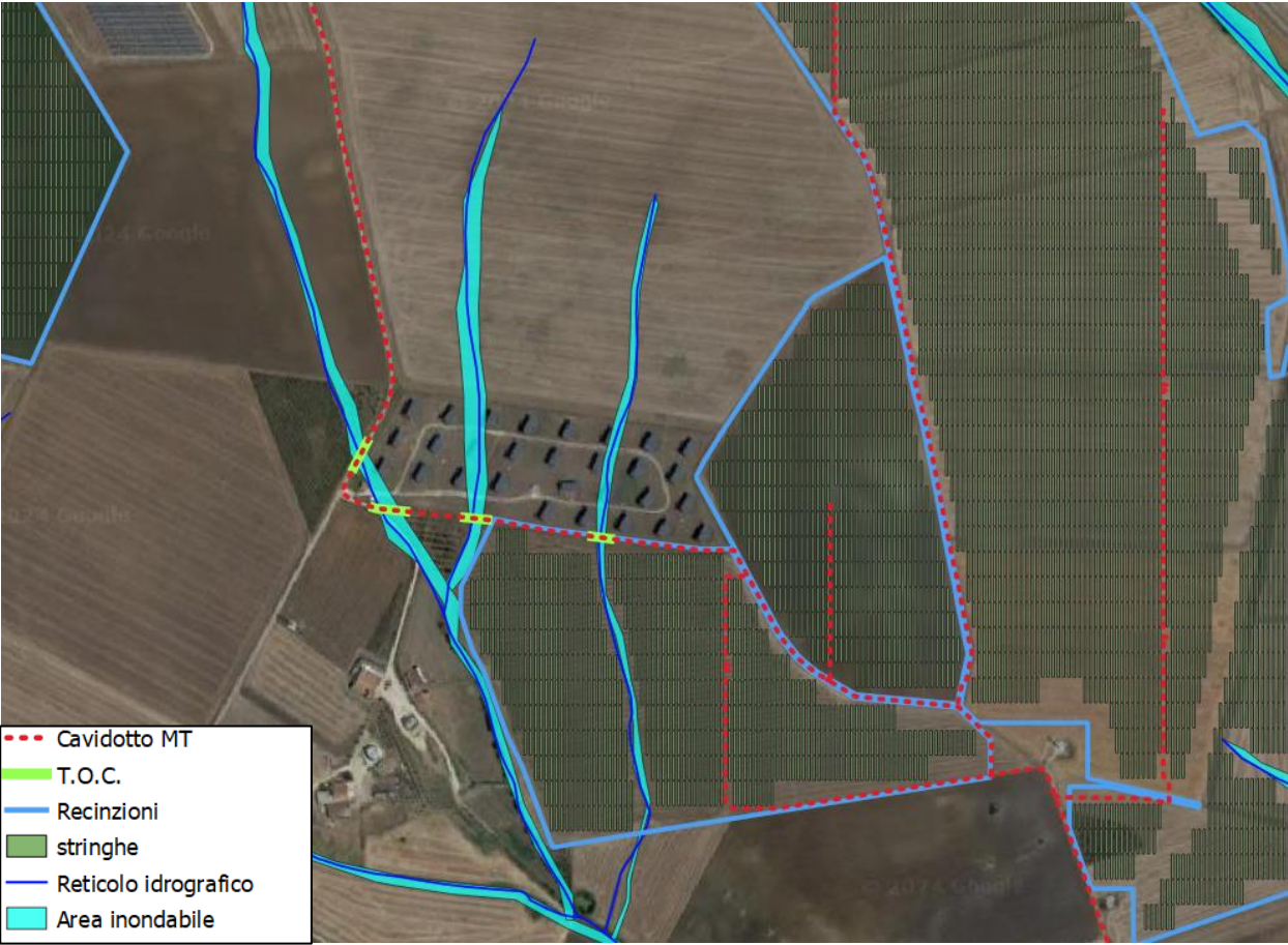
Attraversamento in T.O.C.
