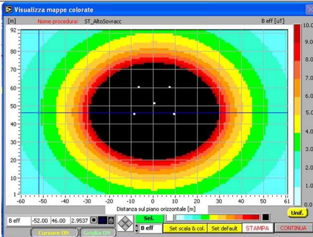
SOSTEGNO A TRALICCIO SINGOLA TERNA 380 kV ALTO SOVRACCARICO TIPO G1: **DPA = 52 m**
