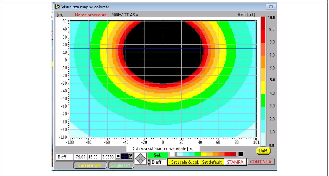
SOSTEGNO A TRALICCIO DOPPIA TERNA 380 kV ALTO SOVRACCARICO TIPO P: **DPA = 79 m**
