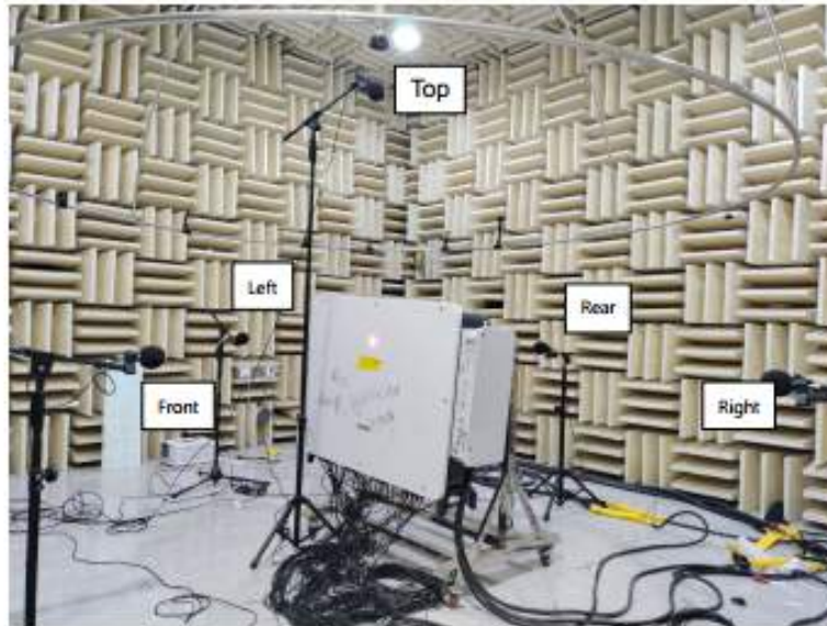
Fig. 3 Sensor Location in the Test
