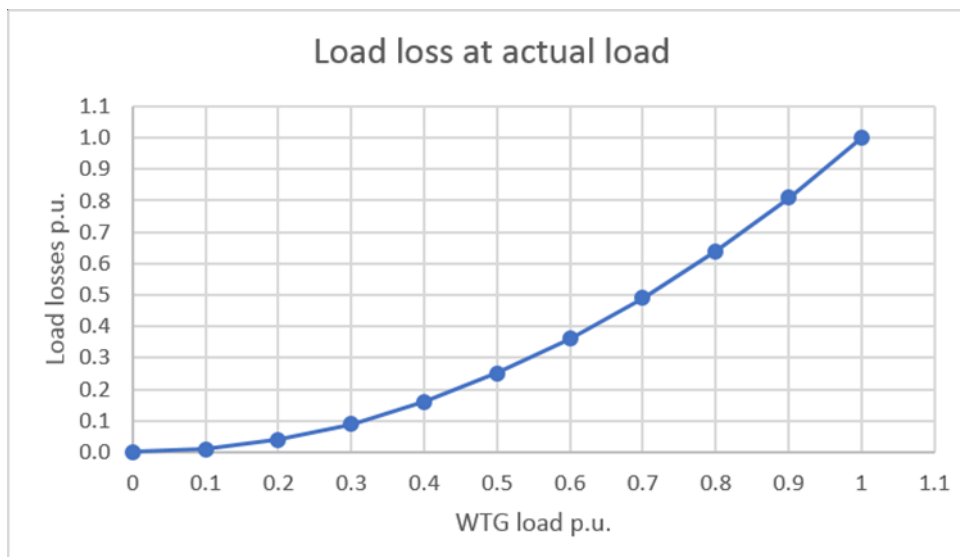
Figure 4-2: Transformer load losses scaling
