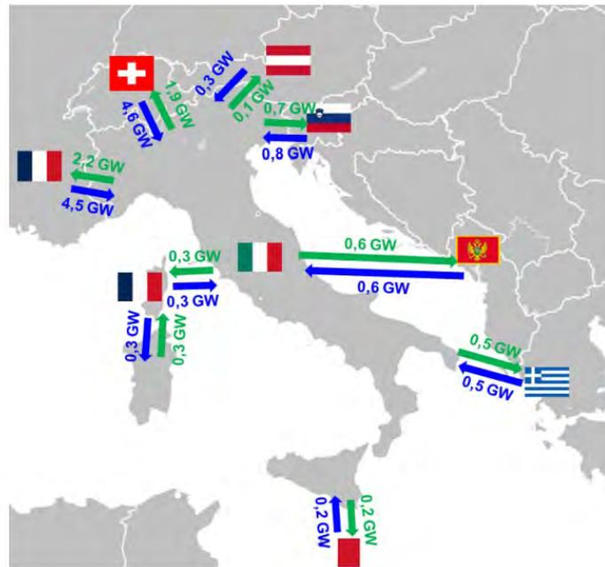
FIGURA 3 - CAPACITÀ DI SCAMBIO TRANSFRONTALIERA IN IMPORT ED EXPORT DELLE INTERCONNESSIONI ESISTENTI
