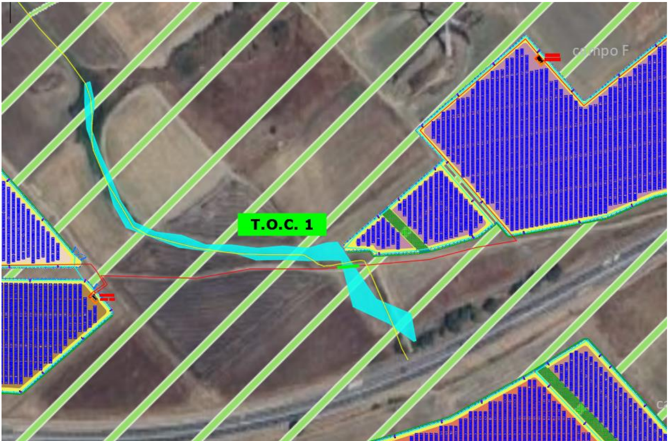
Attraversamento in T.O.C.
