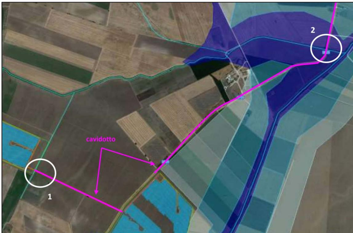
**FIGURA 6 – INTERFERENZA DEL CAVIDOTTO MT INTERRATO CON IL RETICOLO IDRAULICO**
