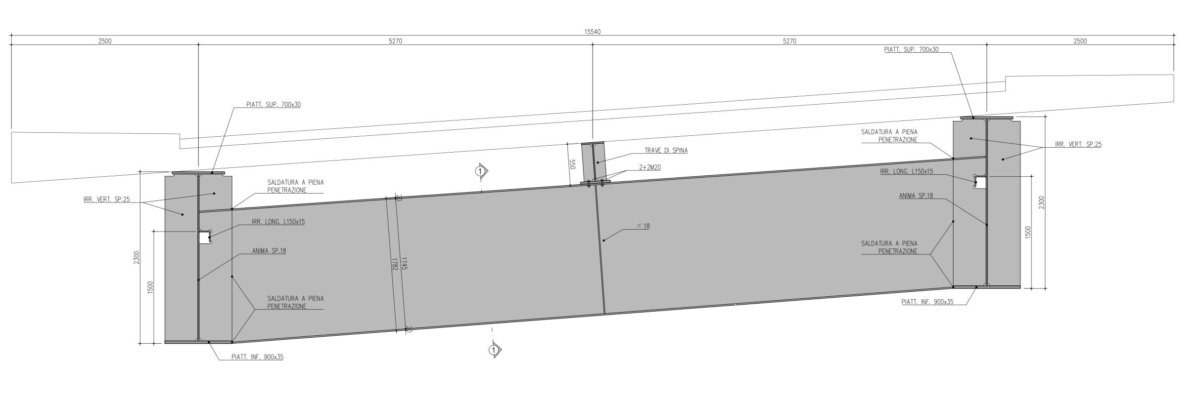
SEZIONE TRASVERSALE SPALLA S2 SCALA 1: 25
