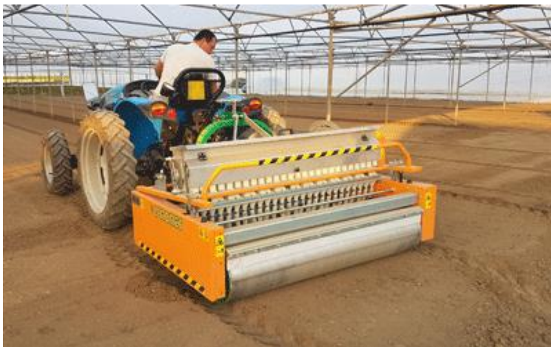
Figura 9 – seminatrice multi-seed (foto Ortomec)
