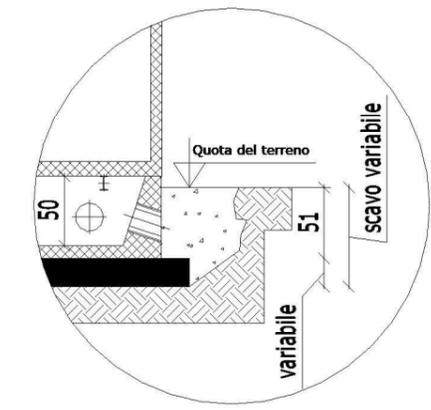
N.B.= ESEGUIRE UNO SCAVO, DI DIMENSIONI IN PIANTA PARI A 0.50 ML. OLTRE IL PERIMETRO DEI PREFABBRICATI, E SUCCESSIVAMENTE REGOLARIZZARE IL PIANO DELLO SCAVO CON PIASTRA IN C.A. DA PROGETTARE A CURA DEL CLIENTE, TENENDO CONTO DI TUTTE LE SOLLECITAZIONI E DELLA NATURA MORFOLOGICA, LITOLOGICA, IDROGEOLOGICA, GEOLOGICA, GEOTECNICA E TOPOGRAFICA DEL TERRENO.
