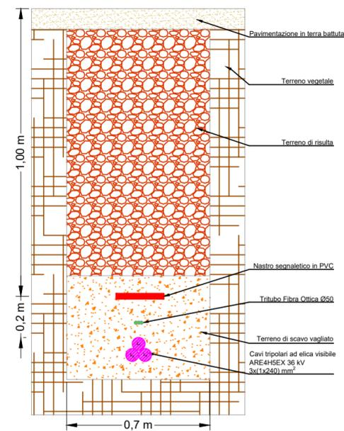
PARTICOLARE DI POSA DI ELETTRDOTTO A 36kV UNA TERNA
