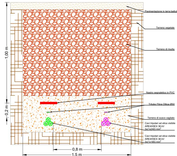
PARTICOLARE DI POSA DI UNA DORSALE A 36 kV IN USCITA
