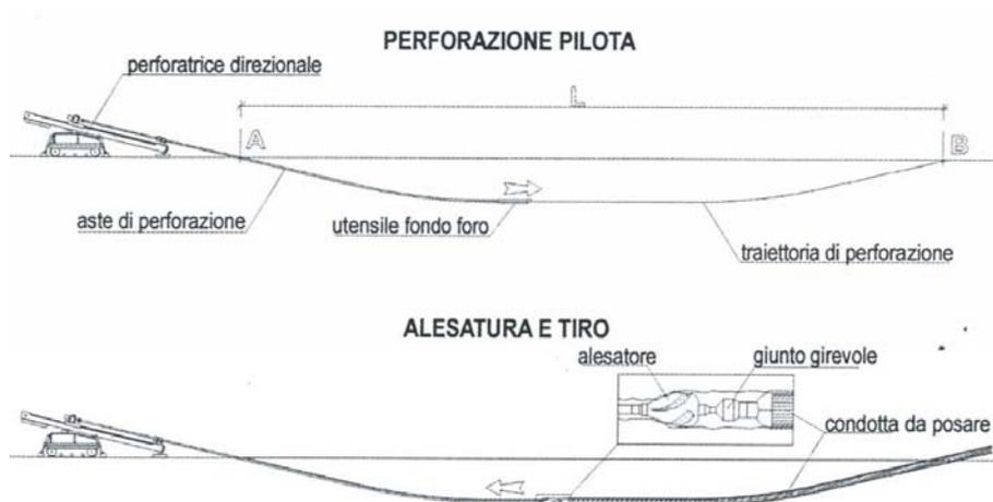
Figura 11-2 - Directional drilling
